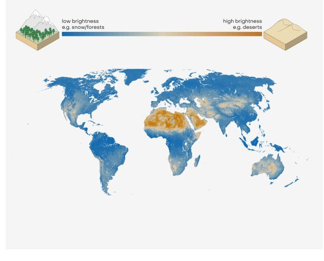
Dark ground surfaces, like forests, will not reflect enough light back towards the satellite sensor, possibly leading to <u>higher uncertainty</u>. As with low sun elevation, this might make it difficult to detect methane absorption. Snow-covered areas also appear mostly dark in the shortwave infrared wavelengths used to detect methane. This effect can be easily seen over tropical forests and snow-covered
