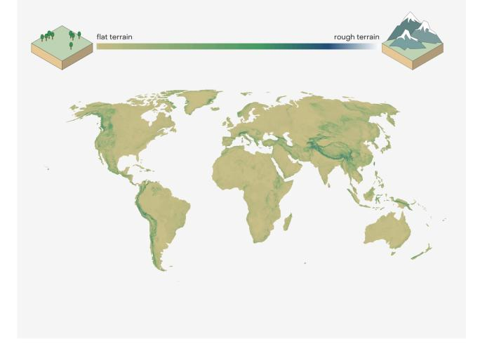
Some satellites find it challenging to estimate methane in regions with <u>mountainous terrain</u>. The uneven ground in such regions will create shadows in part of the observed scene, making it hard to interpret the amount of light that reaches the satellite. As light reflects off different parts of the uneven terrain, it will reach the satellite having passed through different parts of the atmosphere,
