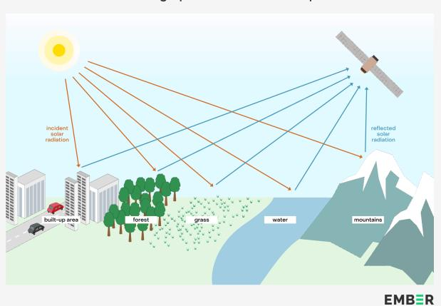
Satellite instruments observe the sunlight reflected from the surface of the earth and search for the fingerprint of methane absorption
