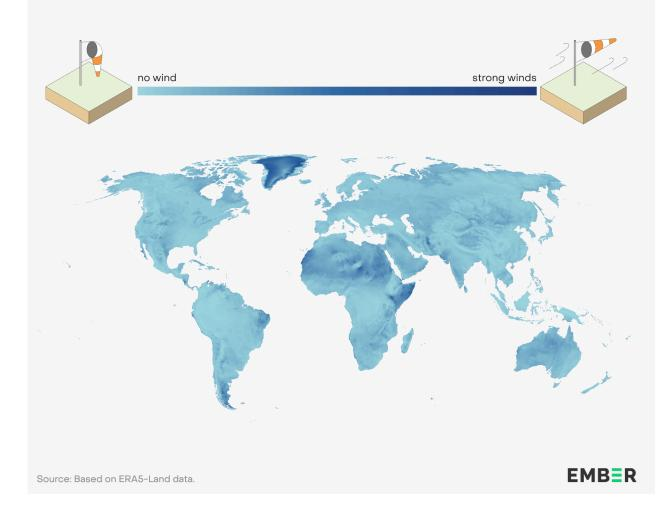
Strong winds can quickly disperse methane far from its source, reducing local concentrations and thus making it harder for a satellite to distinguish the plume from background methane concentration. While a certain amount of wind is needed for plume formation and thus plume quantification, in general, higher wind speeds are associated with <u>higher detection thresholds</u>.
